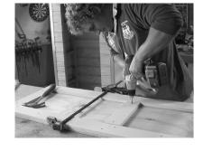
STEP 7 Cut door (R) to size, then, taking size from the door, prepare door stiles and rails (S,T). For an internal frame, screw onto back of door, and if frame is to be exposed, screw on from the back – the frame helps stop door from warping.
